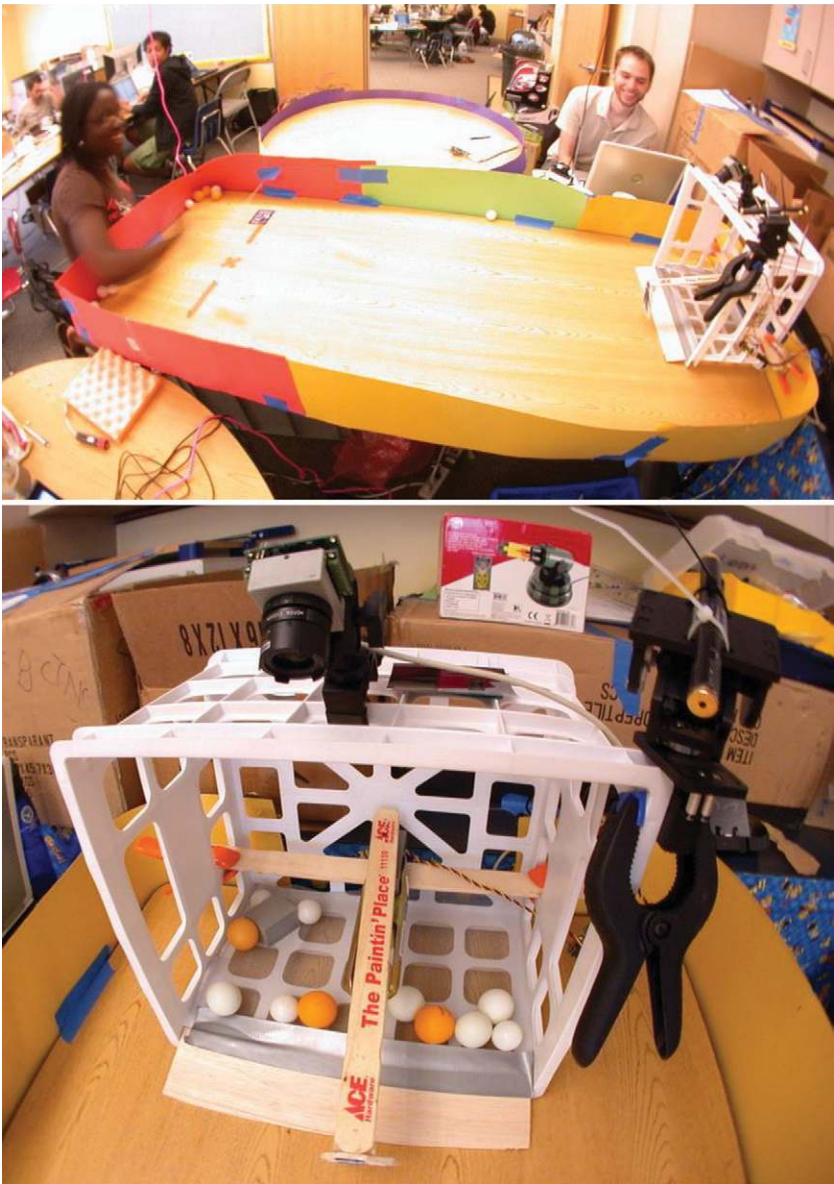
Figure 14.5 Neuromorphic goalkeeper at the 2013 Workshop on Neuromorphic Engineering in Telluride. (Top) Fopefolu Folowosele (left) tests the neuromorphic goalkeeper (right). Other students and their projects can be seen in the background. (Bottom) Delbrück's DVS camera directs a paddle at the end of a paint mixing stick. The goalkeeper is much faster than the students and saves every shot on goal. I also tried and failed to make a goal. Courtesy of Tobias Delbrück.
